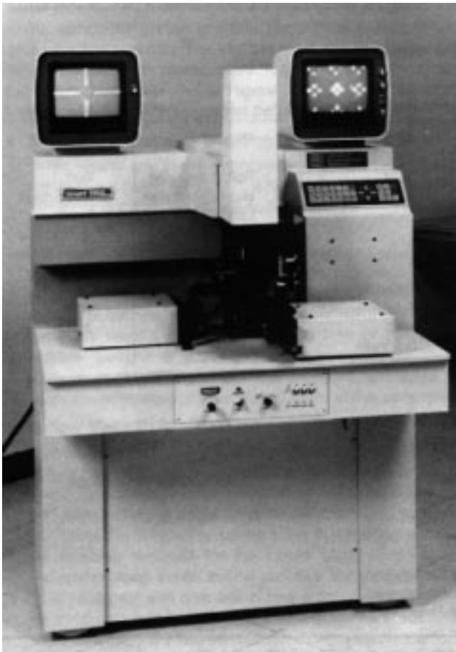
Figure 6. The Machine Shown Above Automatically Dispenses Small Dots of Epoxy and Picks and Places the Beam Lead Devices onto the epoxy dots
